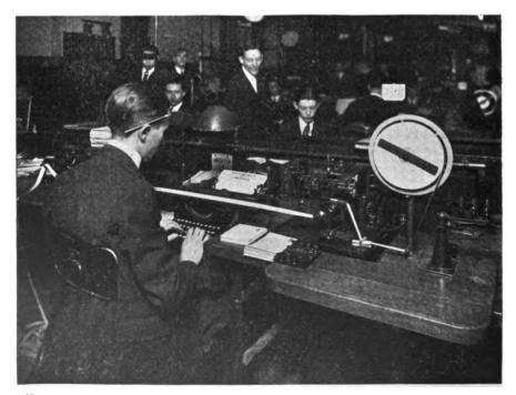
Here a message is being received on a direct New York-London cable. The operator types cablegrams directly from a paper tape running continuously before him Digitized by Google
