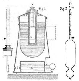
Fig. 1-M. Boland's "Aleurometre." A, closed cylinder, in oopper. It is composed of two principal parts screwed together. t. copper tube, graduated into 25 spaces, from 25 to 50. H, oil bath. T, thermometer for ascertaining the temperature of the boller. Fig. 2-M. Robine's "Appreciateur."
