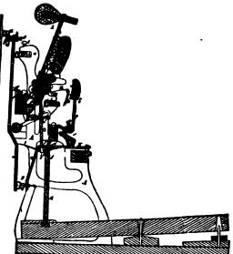
In the above cut, A denotes the metallic frame for supporting the different wooden rails B, C, D and E of the action. The upper of such rails, which is the damper-check rail, is sustained by notched standards a, extending up from the remainder of the frame. These standards are recessed, as represented at b, to receive the said rail, which is held in place by clamp screws c c, arranged in the standards so as to screw down upon the rail.
